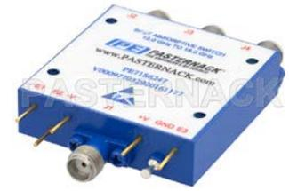
Absorptive SP3T PIN Diode Switch Operating From 12 GHz to 18 GHz Up to 0.1 Watts (+20 dBm) and Field Replaceable SMA
