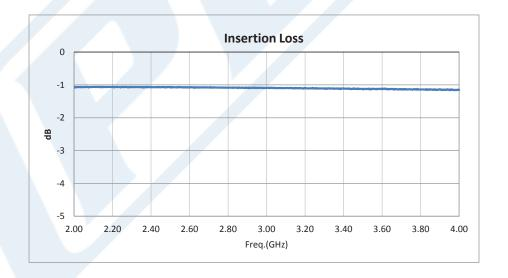
Click the following link (or enter part number in "SEARCH" on website) to obtain additional part information including price, inventory and certifications: Absorptive SPDT PIN Diode Switch Operating From 2 GHz to 4 GHz Up to +27 dBm and Field Replaceable SMA PE71S6208
