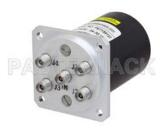
SP4T Electromechanical Relay Normally Open Switch, DC to 40 GHz, 3W, 28V, Indicators, TTL, Diodes, 2.92mm
