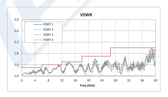
Click the following link (or enter part number in "SEARCH" on website) to obtain additional part information including price, inventory and certifications: SP4T Electromechanical Relay Normally Open Switch DC to 40 GHz, 2.92mm, 3 Watts, 12V Control PE71S6134
