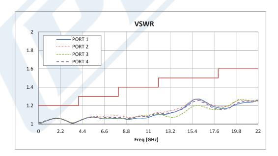
Click the following link (or enter part number in "SEARCH" on website) to obtain additional part information including price, inventory and certifications: SP4T Electromechanical Relay Normally Open Switch DC to 22 GHz, SMA, 20 Watts, 28V Control, Indicators, TTL, Diodes PE71S6129
