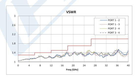
Click the following link (or enter part number in "SEARCH" on website) to obtain additional part information including price, inventory and certifications: Transfer Electromechanical Relay Failsafe Switch DC to 40 GHz, 2.92mm, 5 Watts, 12V Control PE71S6118
