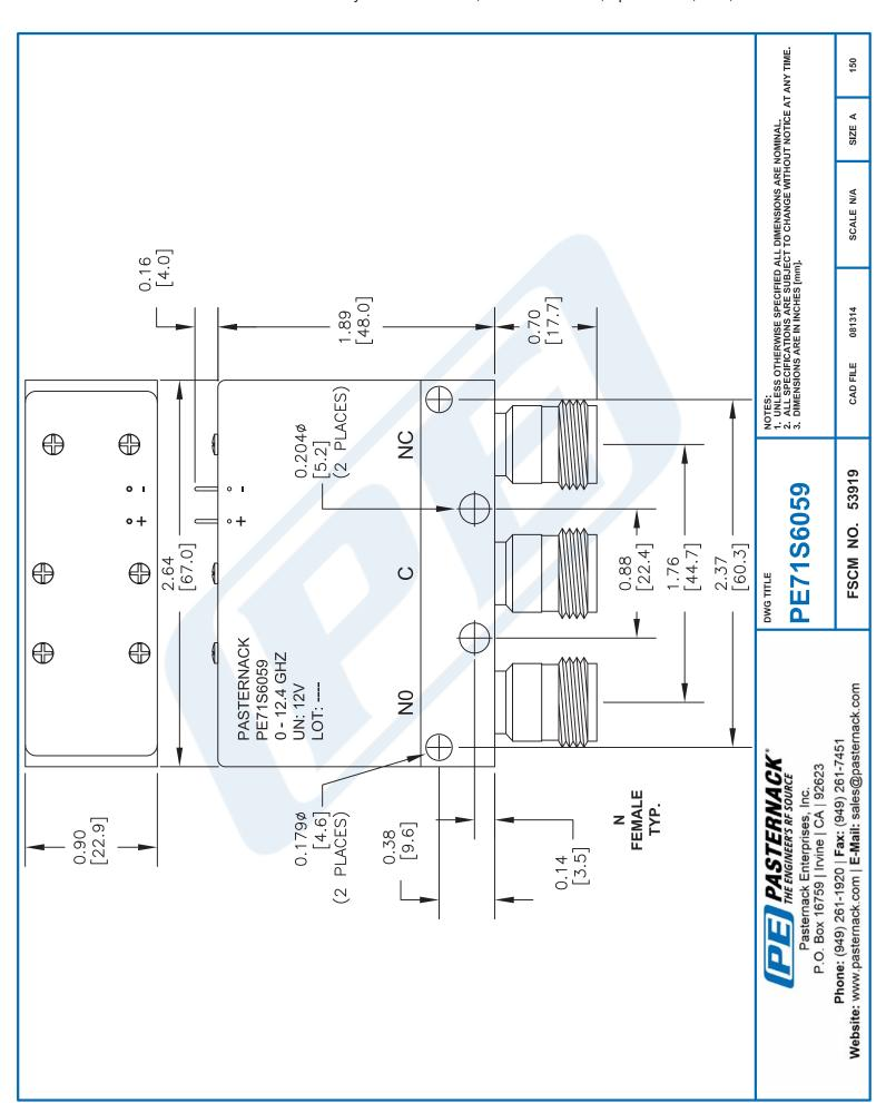
**PE71S6059 CAD Drawing**SPDT Electromechanical Relay Failsafe Switch, DC to 12.4 GHz, up to 700W, 12V, N
