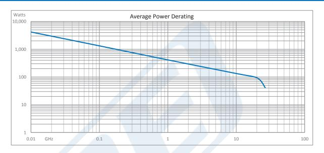
Click the following link (or enter part number in "SEARCH" on website) to obtain additional part information including price, inventory and certifications: SPDT Electromechanical Relay Failsafe Switch, DC to 18 GHz, up to 240W, 28V, SMA PE71S6052
