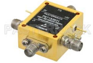
SPDT PIN Diode Switch Operating From 2 GHz to 40 GHz Up to +27 dBm and 2.92mm
