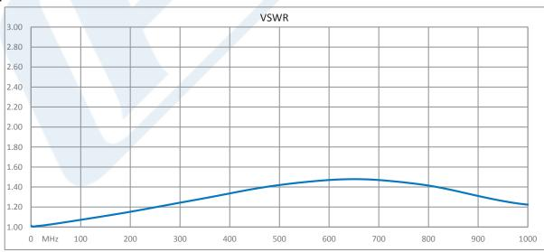
Click the following link (or enter part number in "SEARCH" on website) to obtain additional part information including price, inventory and certifications: A/B Coaxial Electromechanical Relay Switch, DC to 1,000 MHz, 5W, 12V, BNC PE7100
