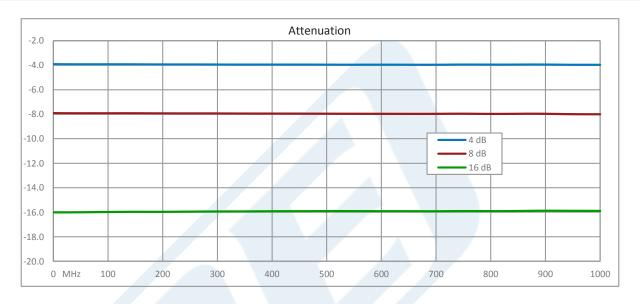
6 Bit Relay Controlled Programmable Attenuator, 31.5 dB Up to 1,000 MHz, 0.5 dB Steps, +12V, SMA Female from Pasternack Enterprises has same day shipment for domestic and International orders. Our RF, microwave and millimeter wave products maintain a 99.4% availability and are part of the broadest selection in the industry.
