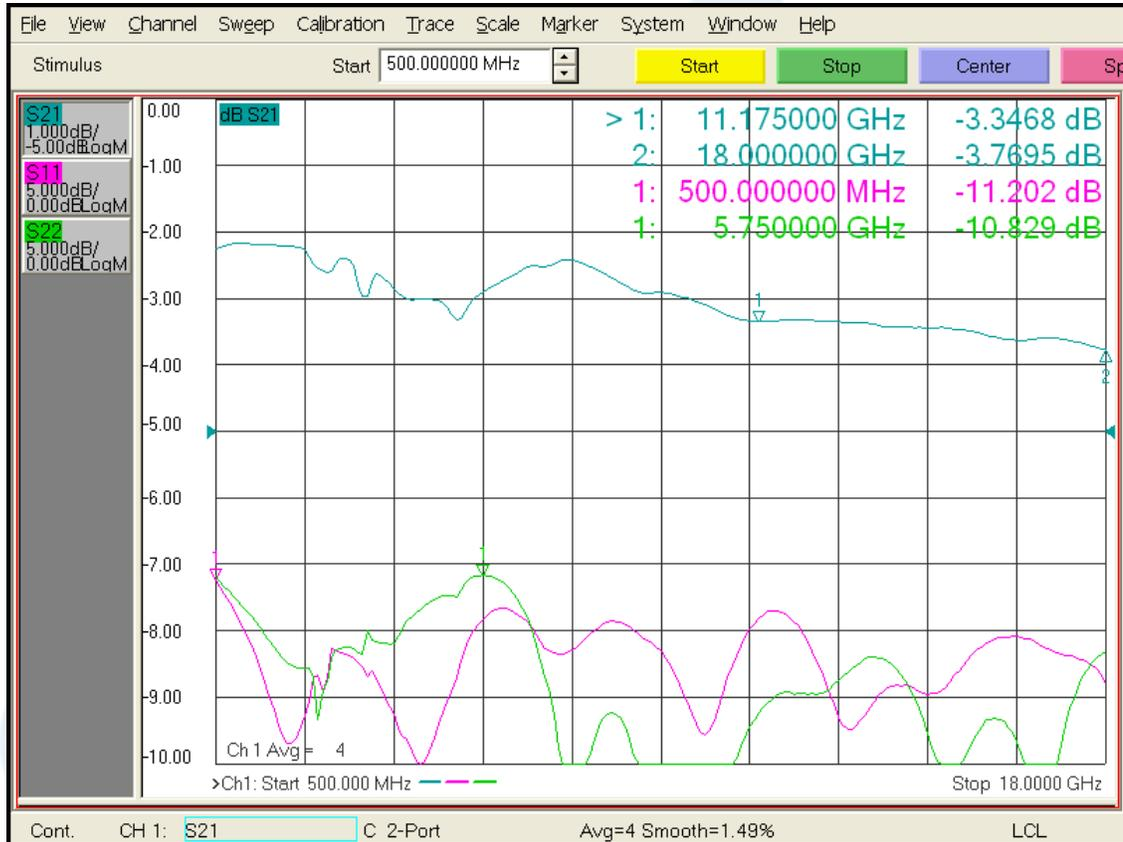
Click the following link (or enter part number in "SEARCH" on website) to obtain additional part information including price, inventory and certifications: [0 to 60 dB Voltage Variable Attenuator, PIN Diode, 500 MHz To 18 GHz, Rated To 0.1 Watts, SMA PE70A2900](#)
