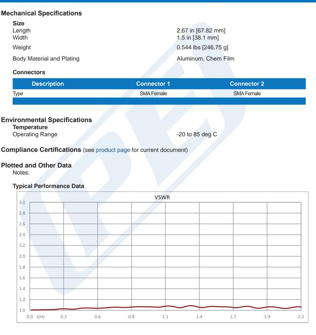
Click the following link (or enter part number in "SEARCH" on website) to obtain additional part information including price, inventory and certifications: 0 to 70 dB Rotary Step Attenuator, SMA Female to SMA Female With 10 dB Step Rated to 2 Watts Up to 2.2 GHz PE70A1023
