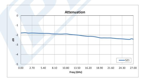
Click the following link (or enter part number in "SEARCH" on website) to obtain additional part information including price, inventory and certifications: 2 dB Fixed Attenuator, SMA Male to SMA Female Passivated Stainless Steel Body Rated to 2 Watts Up to 26 GHz PE7087-2
