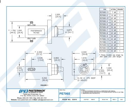
0 to 20 dB Rotary Continuously Variable Attenuator, SMA Female To SMA Female Rated To 5 Watts From 2 GHz To 4 GHz from Pasternack Enterprises has same day shipment for domestic and International orders. Our RF, microwave and millimeter wave products maintain a 99% availability and are part of the broadest selection in the industry.
