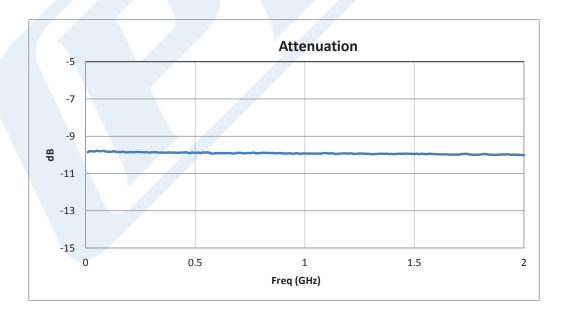
Click the following link (or enter part number in "SEARCH" on website) to obtain additional part information including price, inventory and certifications: 10 dB Fixed Attenuator, BNC Male to BNC Female Brass Nickel Body Rated to 1 Watt Up to 2 GHz PE7000-10
