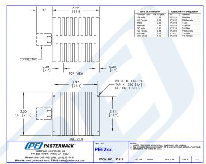
50 Watt RF Load Up To 18 GHz With SMA Female Input Square Body Black Anodized Aluminum Heatsink from Pasternack Enterprises has same day shipment for domestic and International orders. Our RF, microwave and millimeter wave products maintain a 99% availability and are part of the broadest selection in the industry.
