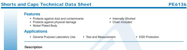
Pasternack's PE6136 connector dust cap has a TNC interface and a female gender. Our TNC female dust cap is a shorting design with a nickel plated body to ensure durability. The Pasternack shorting TNC connector cap comes with a 4 inch chain and is part of over 40,000 RF, microwave and millimeter wave products that ship the same day.
