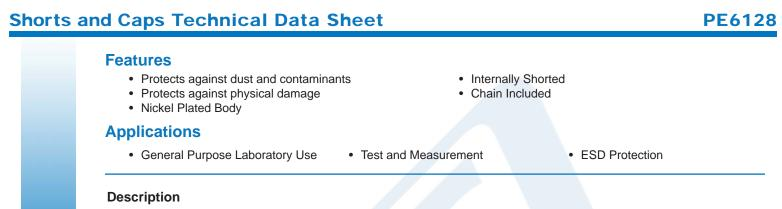
Pasternack's PE6128 connector dust cap has a BNC interface and a female gender. Our BNC female dust cap is a shorting design with a nickel plated body to ensure durability. The Pasternack shorting BNC connector cap comes with a 4 inch chain and is part of over 40,000 RF, microwave and millimeter wave products that ship the same day.
