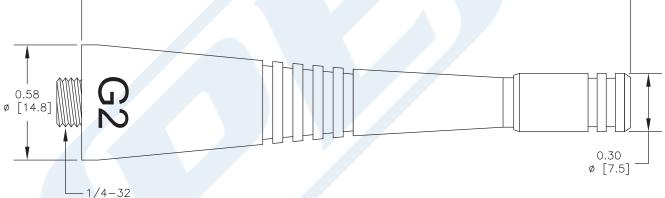
Click the following link (or enter part number in "SEARCH" on website) to obtain additional part information including price, inventory and certifications: Whip Antenna Operates From 880 MHz to 960 MHz With a Typical 0 dBi Gain MX Input Connector IP67 Rated PE51164
