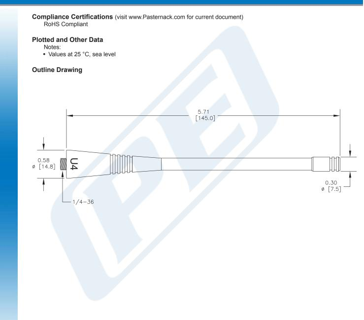
Click the following link (or enter part number in "SEARCH" on website) to obtain additional part information including price, inventory and certifications: Whip Antenna Operates From 470 MHz to 512 MHz With a Typical 0 dBi Gain SMA Female Input Connector IP67 Rated PE51161
