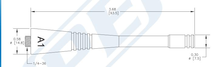
Click the following link (or enter part number in "SEARCH" on website) to obtain additional part information including price, inventory and certifications: Whip Antenna Operates From 698 MHz to 780 MHz With a Typical 0 dBi Gain SMA Female Input Connector IP67 Rated PE51157
