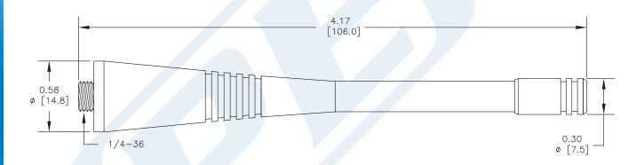
Click the following link (or enter part number in "SEARCH" on website) to obtain additional part information including price, inventory and certifications: Whip Antenna Operates From 698 MHz to 870 MHz With a Typical 2 dBi Gain SMA Female Input Connector IP67 Rated PE51152
