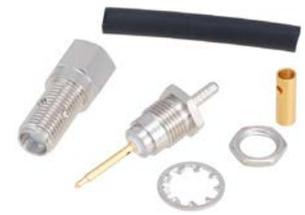
RP-SMA Female Bulkhead Mount Connector Solder Attachment for RG178, RG196, .235 inch D Hole
