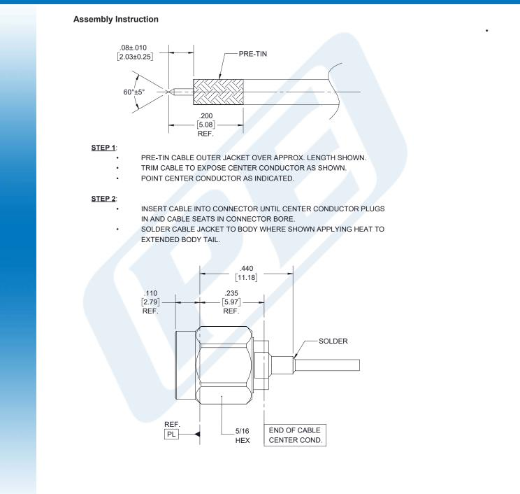
Click the following link (or enter part number in "SEARCH" on website) to obtain additional part information including price, inventory and certifications: 2.92mm Male Connector Solder Attachment for PECX005, PECX006, Low Loss 086 Semi-Rigid PE45485
