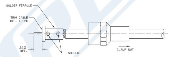
3. SOLDER CONTACT WITH GAP INDICATED AS SHOWN.
