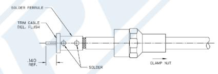
3. SOLDER CONTACT WITH GAP INDICATED AS SHOWN.
