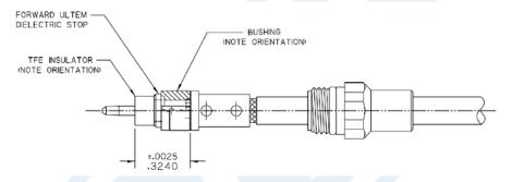
INSERT CABLE/CONTACT SUB-ASSEMBLY INTO CONNECTOR UNTIL SEATED AND TIGHTEN CLAMP NUT TO 35-45 IN-LBS.
