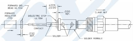
INSERT CABLE/CONTACT SUB-ASSEMBLY INTO CONNECTOR UNTIL SEATED AND TIGHTEN CLAMP NUT TO 25-35 IN-LBS.
