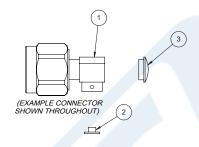
1. STRIP CABLE AS SHOWN, CHAMFER CENTER CONDUCTOR AND DEBURR CABLE
