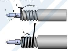
PUSH THE CONNECTOR BODY INTO THE CABLE, UNTIL IT STOPS. SOLDER THE CONNECTOR BODY WITH CABLE.
