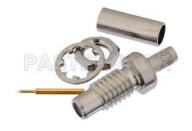
SMC Jack Bulkhead Mount Connector Crimp/Solder Attachment for RG188-DS, RG316-DS, .177 inch D Hole
