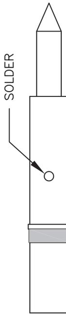
3. SLIDE INSULATOR THROUGH CONTACT UNTIL IT BOTTOMS OUT. INSERT INSULATOR TO BODY UNTIL IT MATES. SOLDER BODY TO CABLE.
