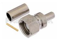
75 Ohm SMC Plug Connector Crimp/Solder Attachment for PE-B150, RG180, RG195
