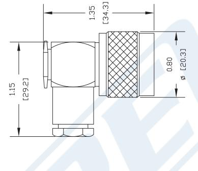
TO DIMENSION SHOWN. DO NOT NICK CENTER CONDUCTOR. TIN CENTER CONDUCTOR. SLIDE ASSEMBLY FORM BRAID OVER CLAMP NUT (4). CUT DIELECTRIC NTO BODY, SOLDER CENTER CONDUCTOR IN PLACE & TIGHTEN CLAMP NUT. SCREW CAP DOWN INTO PLACE. PE4135 REV 1.3
