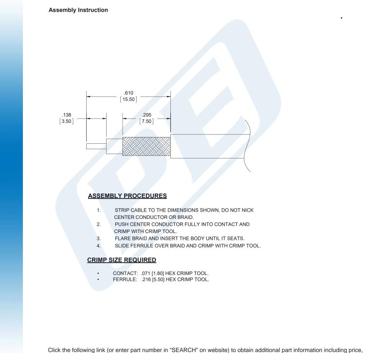
Click the following link (or enter part number in "SEARCH" on website) to obtain additional part information including price, inventory and certifications: BNC Male Connector Crimp/Crimp Attachment for RG58, RG303, RG141, PE-C195, PE-P195, LMR-195, 0.195 inch PE4016
