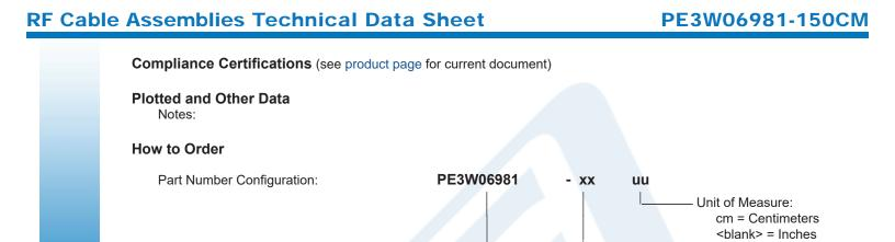
Example: PE3W06981-12 = 12 inches long cable PE3W06981-100cm = 100 cm long cable
