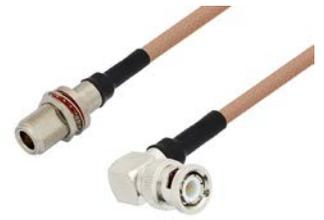
N Female Bulkhead to BNC Male Right Angle Cable 36 Inch Length Using RG400 Coax with HeatShrink, LF Solder
