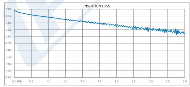
Click the following link (or enter part number in "SEARCH" on website) to obtain additional part information including price, inventory and certifications: Reverse Polarity SMA Male to N Female Bulkhead Cable 48 Inch Length Using RG58 Coax PE3W02336-48
