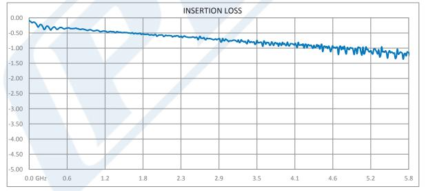
Click the following link (or enter part number in "SEARCH" on website) to obtain additional part information including price, inventory and certifications: SMA Male Right Angle to N Male Right Angle Cable 24 Inch Length Using LMR-195 Coax PE3W00852-24
