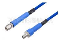
PE-TC195 Series Phase Stable Test Cable SMA Male to SMA Female to 18 GHz 24 Inch Length ,RoHS
