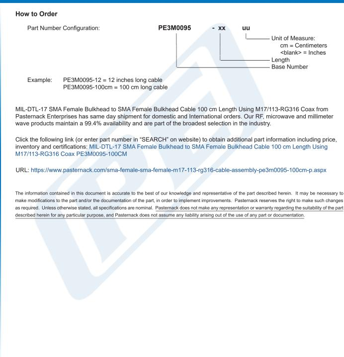
Pasternack Enterprises, Inc. • P.O. Box 16759, Irvine, CA 92623 **Phone:** (866) 727-8376 or (949) 261-1920 • **Fax:** (949) 261-7451 Sales@Pasternack.com • Techsupport@Pasternack.com PE3M0095-100CM CAD Drawing MIL-DTL-17 SMA Female Bulkhead to SMA Female Bulkhead
