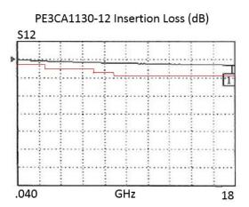
Click the following link (or enter part number in "SEARCH" on website) to obtain additional part information including price, inventory and certifications: SMA Male to Push-On SMA Male Precision Cable 12 Inch Length Using PE-P141 Coax , LF Solder PE3CA1130-12
