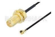
Reverse Polarity SMA Female Bulkhead to UMCX 2.5 Plug Cable 3 Inch Length Using 1.13mm Coax, RoHS
