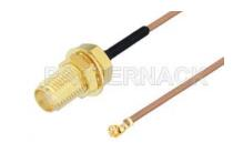
SMA Female Bulkhead to UMCX 2.5 Plug Cable 6 Inch Length Using RG178 Coax, RoHS
