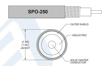
SPO-250 Coax Using Times Microwave Parts PE3C6437-200CM
