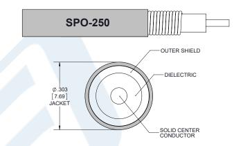
SPO-250 Coax Using Times Microwave Parts PE3C6437-150CM
