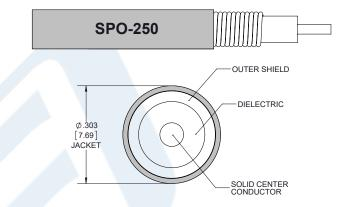
SPO-250 Coax Using Times Microwave Parts PE3C6437-100CM
