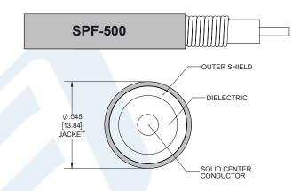
SPF-500 Coax Using Times Microwave Parts PE3C6376-36
