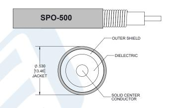
ing SPO-500 Coax Using Times Microwave Parts PE3C6373-48
